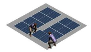
Use a roller to gently roll the component surface to ensure that it is firmly attached. The overall installation effect is as shown in the figure.
